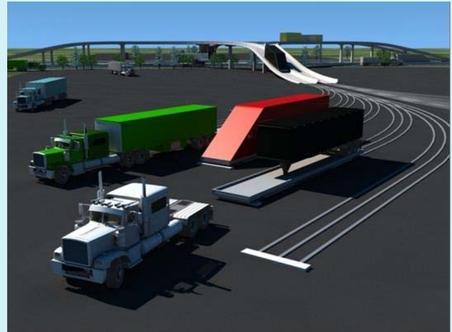
Aerodynamic caps reduce drag; standard 5 th wheel coupling
