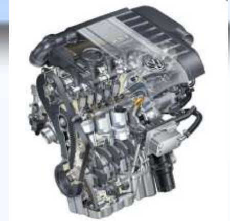
VW Turbocharged GDI Engine
